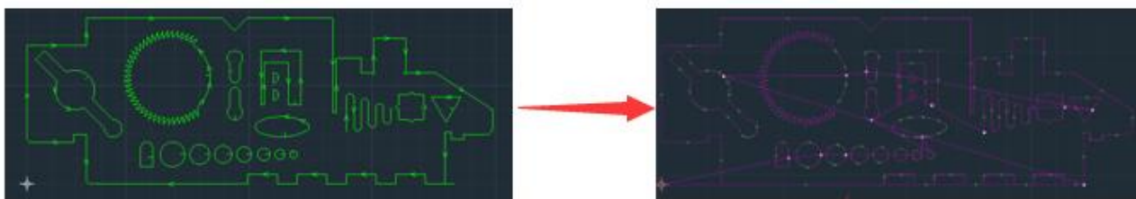
Error measurement(The purple path is feedback path from encoder)
